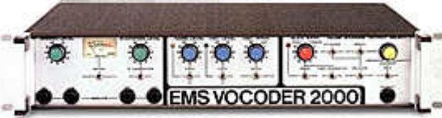
fig. 138 The EMS Vocoder 2000. voice synthesiser
