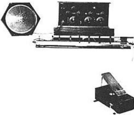
fig. 37 A very early model of the Trautonium
