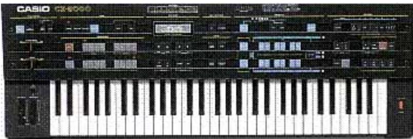
Two CZ-101s with full size keys and an onboard real-time & simple step-edit sequencer. mono output, built in chorus and a cassette interface
