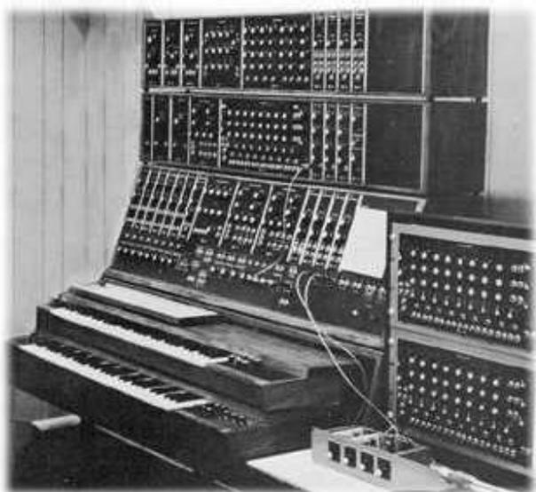
fig. 107 Modular Moog Synthesiser c1967
