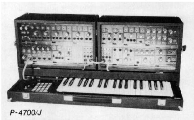
fig. 126 The PAiA P4700/J Synthesizer with built in sequencer
