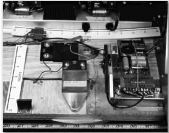
fig. 68 The pressure sensitive devices on the 1971 Sackbut were considerably refined over those of 1948
