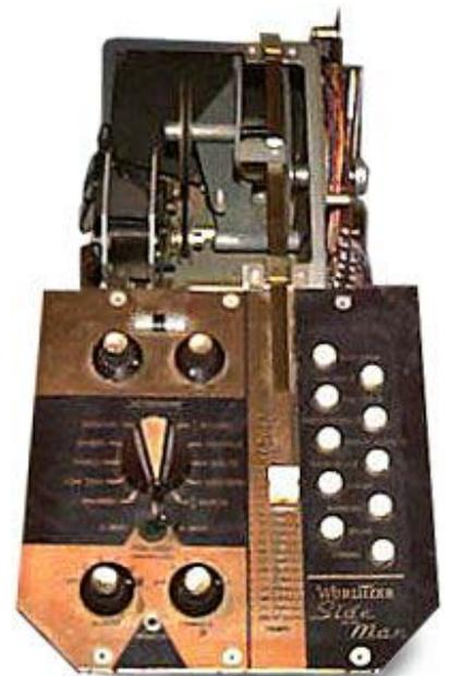
**fig. 102 The top panel of the Sideman showing (L-R) pattern select control, tempo slider and manual triggers**
