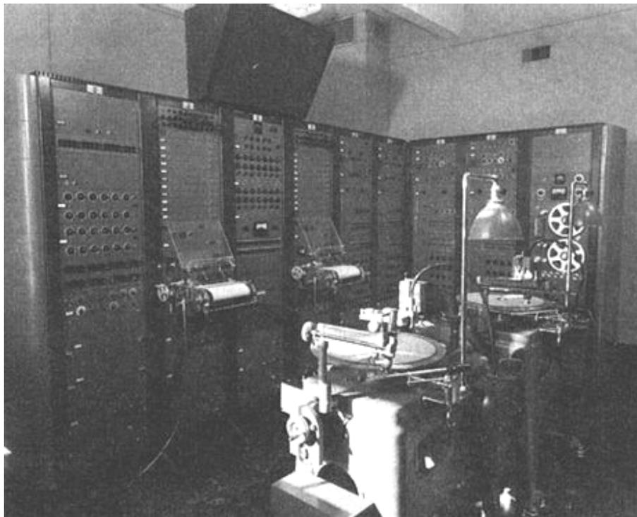
**fig. 88 The RCA mkII showing the laquer disk cutters**
