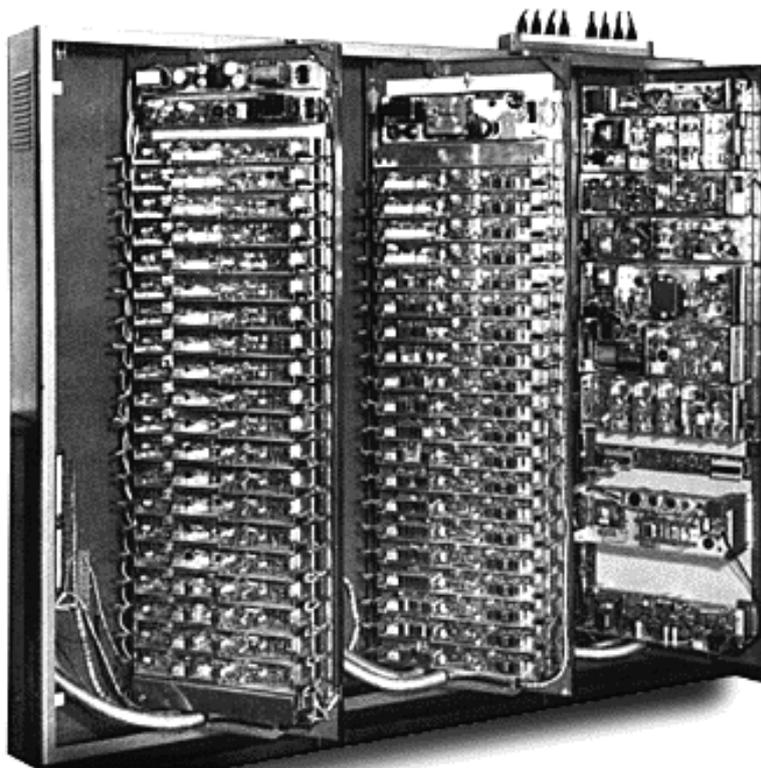
**fig. 95 A Siemens Vocoder opened to show circuits**
