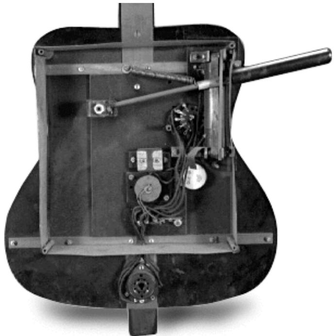
fig. 44 Rear view of the Theremin Cello shows the volume control and tone generator.
