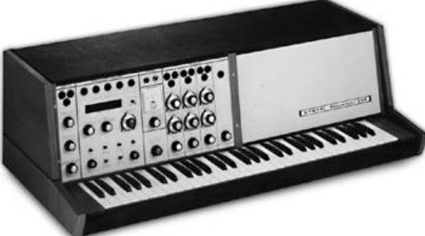
fig. 135 EMS Synthi Sequencer 256. 256 Event x 42 bit Memory sequencer (1971)
