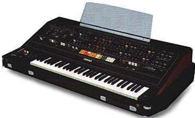
Fig. 149 The Yamaha CS80 polyphonic Synthesiser
