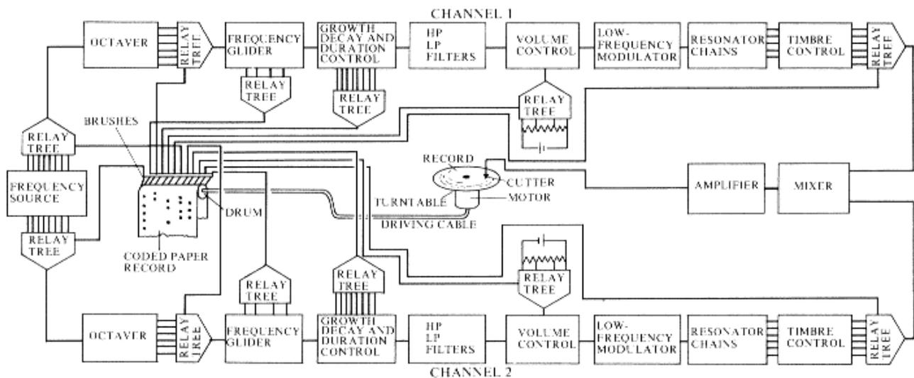
**fig. 83 A diagram of the RCA MkII showing hard disk recording and paper roll programmer.**
