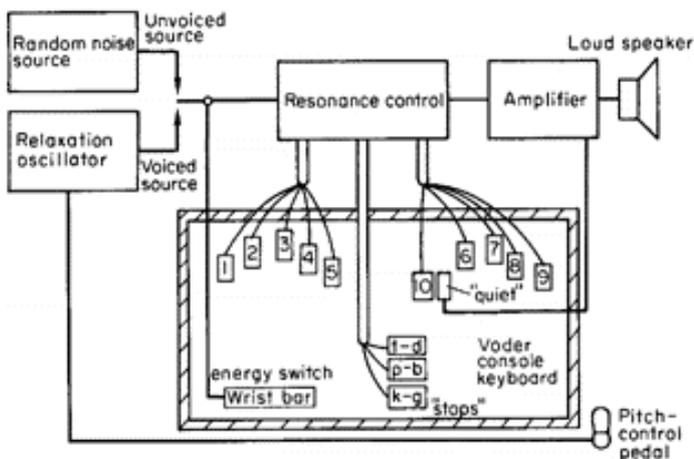
Fig. 53 Diagram of the "Voder"
