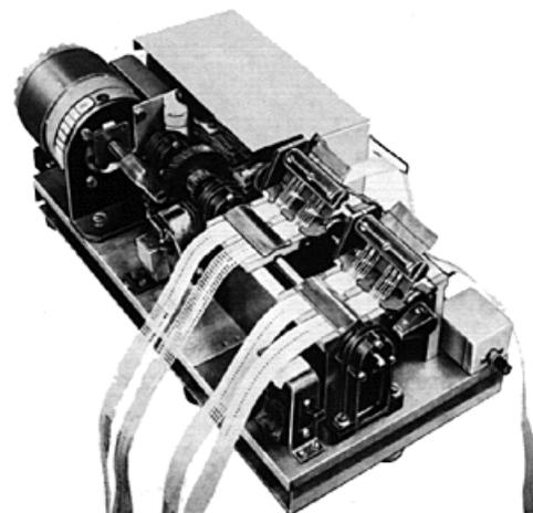
fig. 99 The punch-paper strip controller
