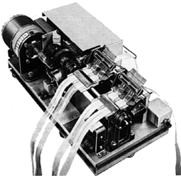
fig. 94 The Siemens punch-tape control mechanism
