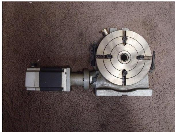
Figure 4-8 Optional Fourth Axis Rotary Table
