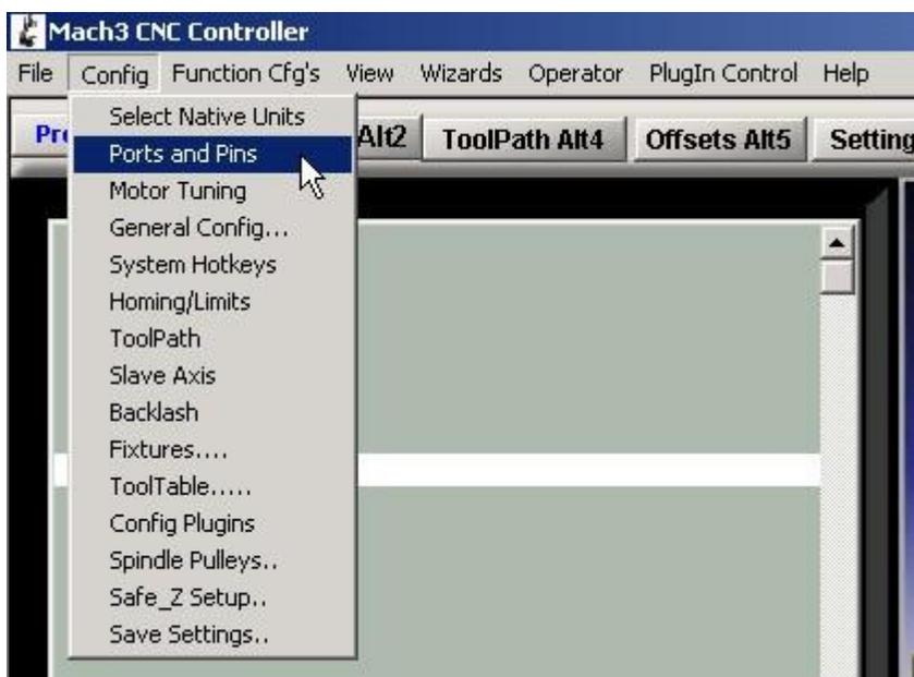
Figure 5-18 SELECTING THE PORTS AND PINS DIALOG FROM THE CONFIG MENU
