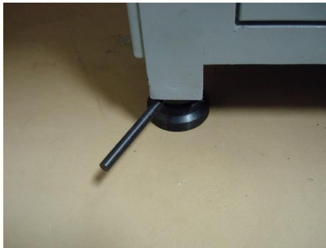
Figure 3-77 Leveling Stand Adjustment Pads
