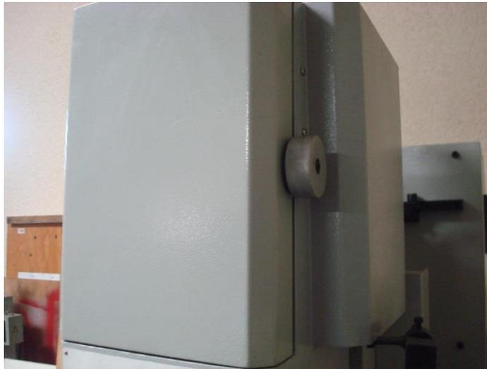
Figure 4-6 Spindle Motor Access/Closure Knob
