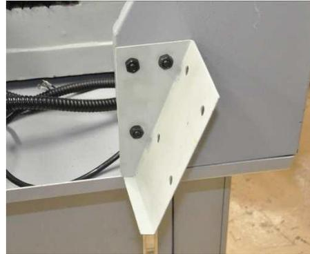
Figure 3-63 Rear Right Shroud Bracket
