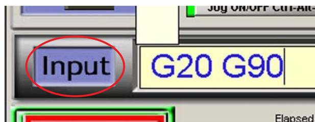
Figure 5-33 MANUALLY ENTERING G20 G90 COMMANDS
