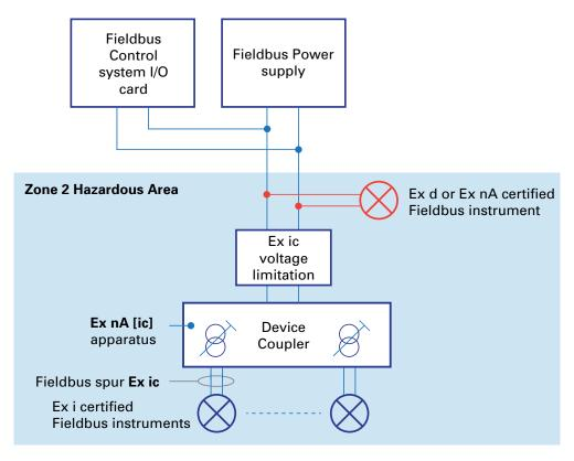
A benefit of defining the trunk as Ex nA is that Ex d or Ex nA field devices can also be connected to the segment
