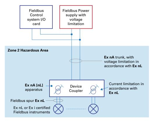
With Ex nL, the fieldbus application used the power supply's inherent voltage limitation
