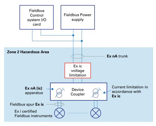
With Ex ic, a separate voltage limiter is inserted to avoid an ambiguous Ex nA/ic classification for the fieldbus trunk
