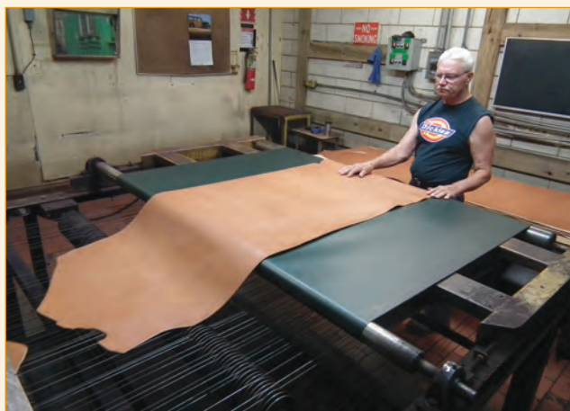
Often leathers are buffed and treated with a sealing coat on the flesh side. To prevent drag marking of the flesh areas, this feed belt (running at the same speed as the feed strings) is used to offer the sides to the spraying operation.
