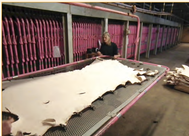
One of the three 180 frame toggle drying units located in a single drying room. Each unit is open sided, and the temperature and relative humidity within the whole drying room is controlled using a single dehumidifying unit to maintain a low-temperature drying operation.
