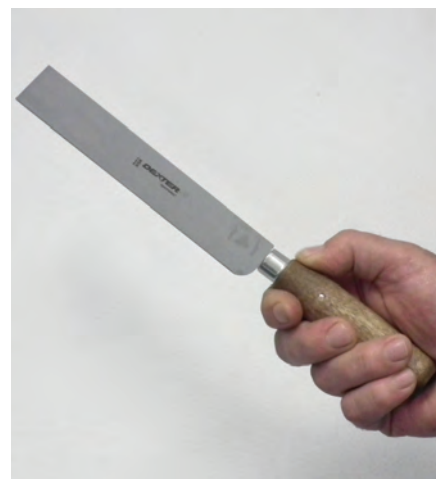
Safety is high on the agenda of this tannery. All of the knives used are either rounded or square cut to avoid a sharp point and the possibility of injury by accidental stabbing.
