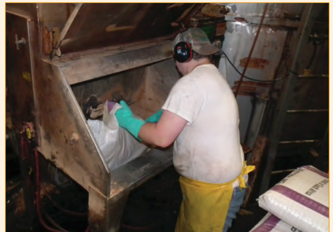
A considerable quantity of vegetable tanning agent is required in the preparation of tanning solutions. Each bag is cut and emptied into this dispensing unit that incorporates a powerful air suction unit to avoid any release of vegetable tanning dust into the air.
