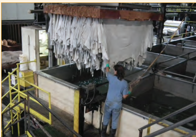
Sides are hung within these hanging frames, then manipulated by hoist into the first of the pits as part of the tanning process.
