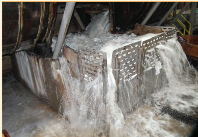
Sides after deliming and preparation for vegetable tanning are discharged from the paddle base into stainless steel dumpsters. The sides of these containers are raised to retain the pieces and allow fast water removal. These sections are removed as required and ease the stacking down of the sides.
