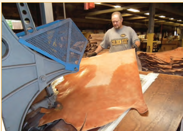
Glazing as a final stage of manufacture of heavy substance aniline drum stuffed leathers.
