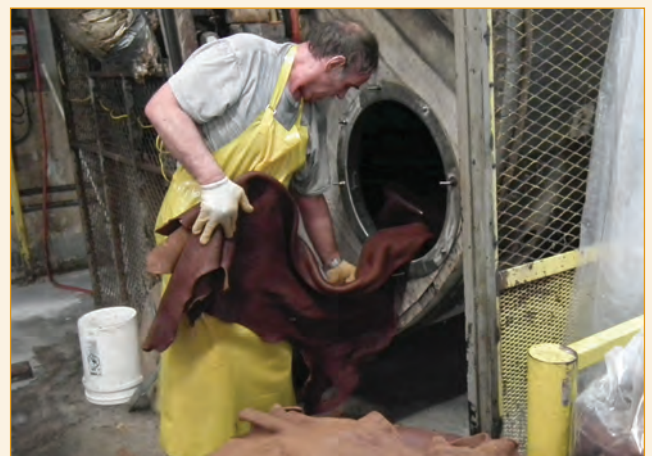
50% of the leathers produced are dyed to shade, samm/set, then drum stuffed with hot waxes and grease. Traditional side loading drums are used for this operation.
