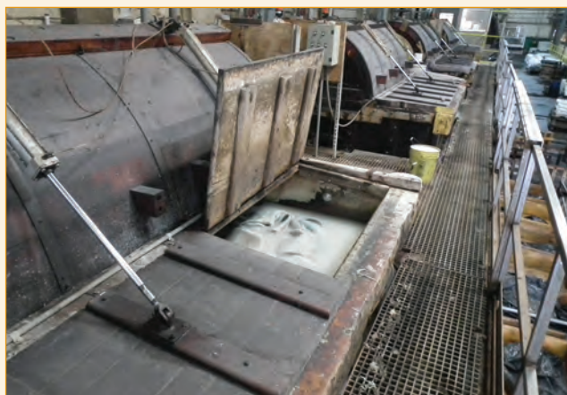
The deliming processes take place in a row of four elevated paddles. The hides are lifted by forklift in a container to the service walkway. The safety guard slides on the guard rail slides to one side to enable access to the load as in turn the container fills the opening.
