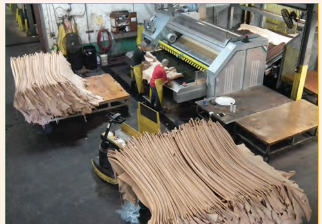
Hides are rinsed and drained, then detached from the frames used within the tanning process being and offered to the setting operation.
