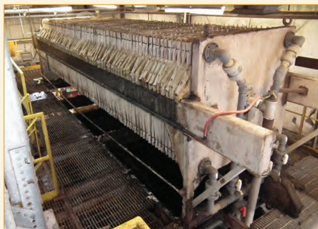
Due to the high organic content from vegetable tannage, the filter press dewater the sludge to approximately 30%. The volume produced is 6m 3 per day, and this is dropped from the mezzanine-mounted press into a truck placed below the press.
