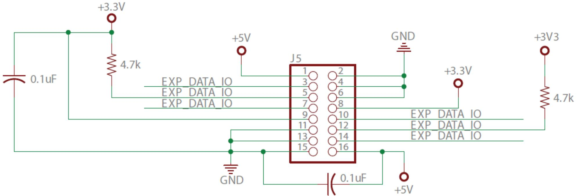
Figure 6-4 Expansion Port Header
