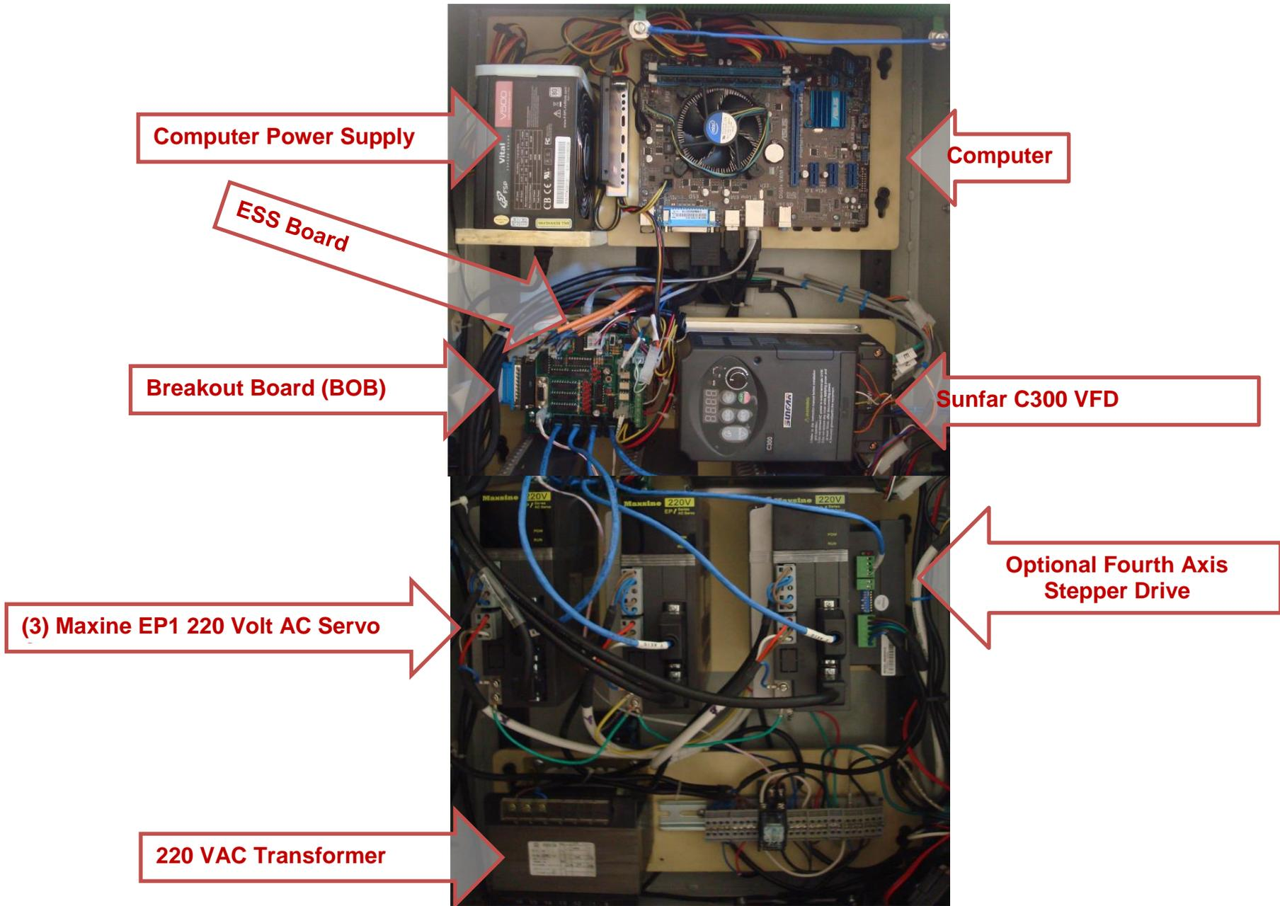
Figure 6-6 Typical Torus PRO Electrical Control Panel
