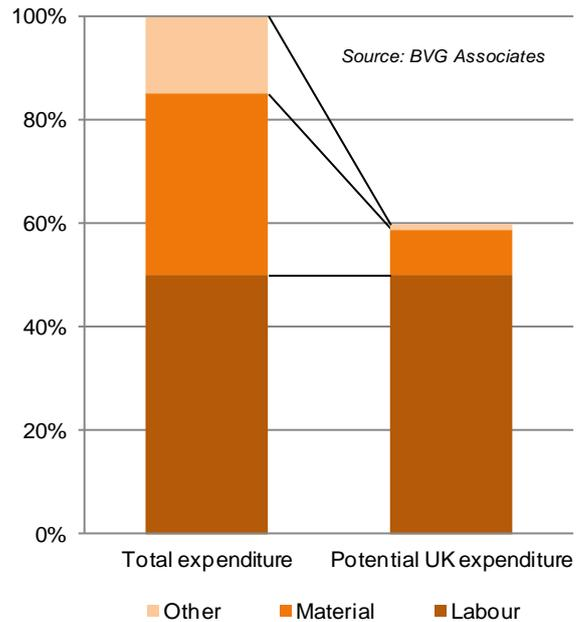
**Figure 4.8 Typical breakdown of total drive train component expenditure and potential UK expenditure.**
