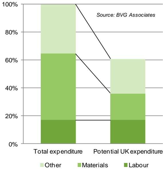
**Figure 5.4 Breakdown of total subsea export cable supply expenditure and potential UK expenditure.**
