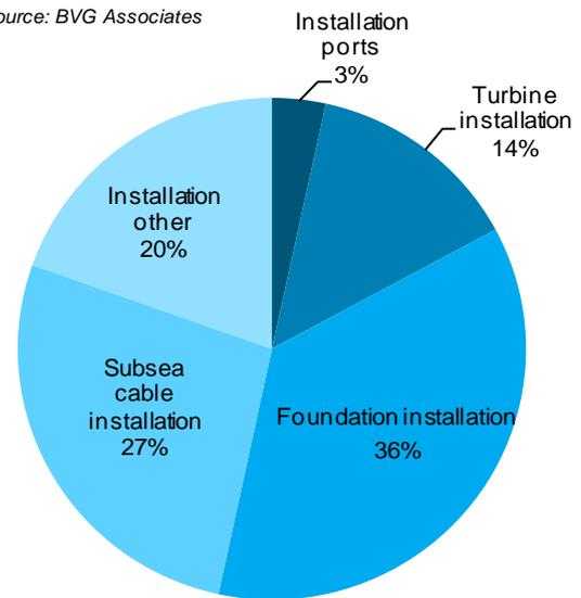
**Figure 6.1 Breakdown of installation and commissioning costs.**
