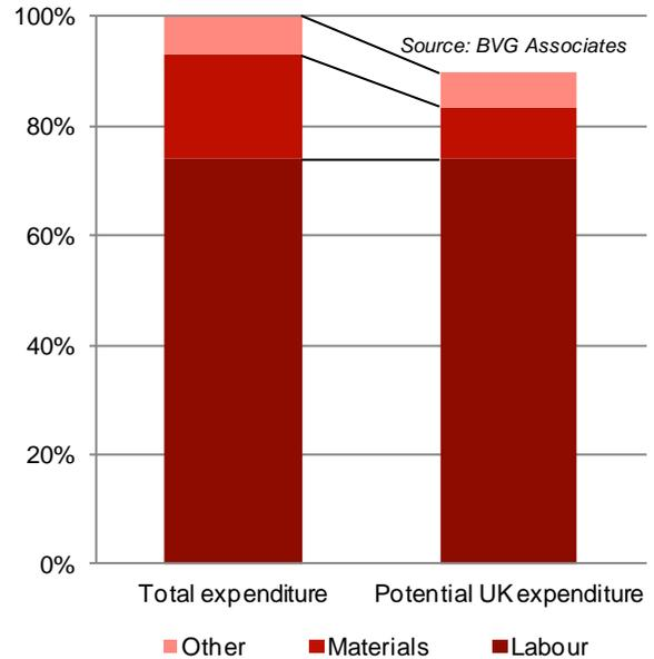
**Figure 3.2 Breakdown of total wind farm design expenditure and potential UK expenditure.**
