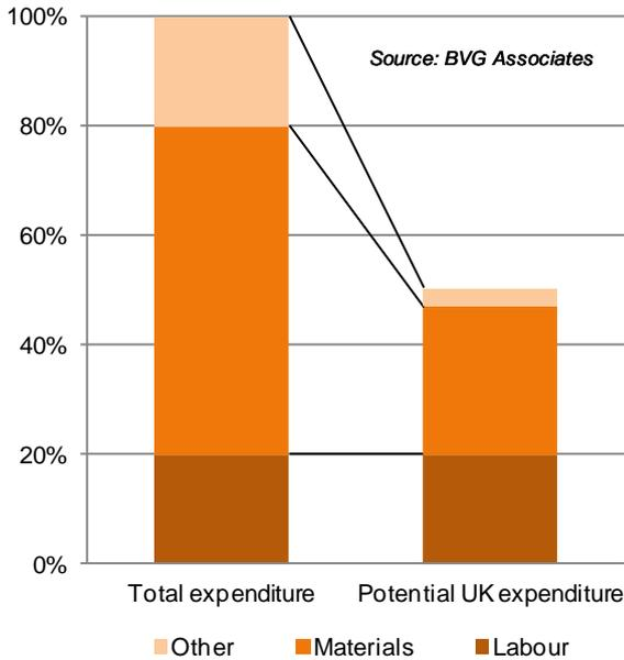
**Figure 4.4 Typical breakdown of total blade supply expenditure and potential UK expenditure.**
