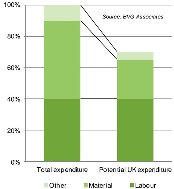
**Figure 5.8 Breakdown of total HVDC substation supply expenditure and potential UK expenditure.**
