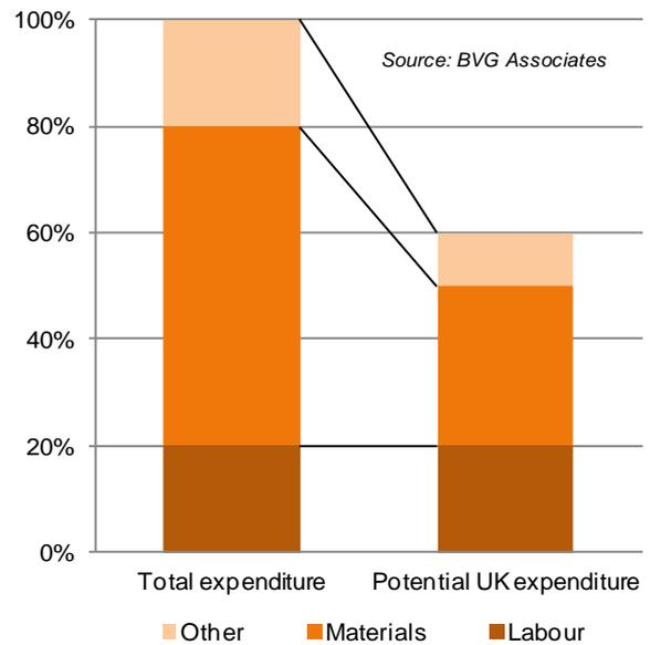
**Figure 4.10 Typical breakdown of total tower supply expenditure and potential UK expenditure.**
