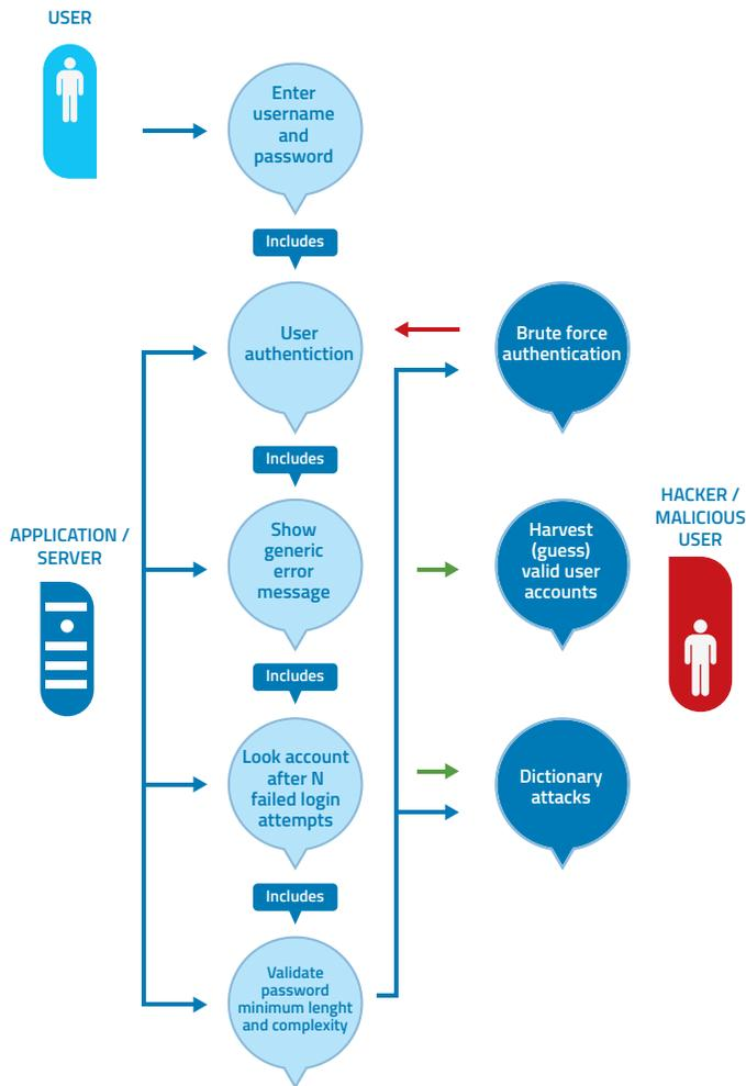
**Step 4:** Elicit The Security Requirements. In this case, the following security requirements for authentication are derived:
