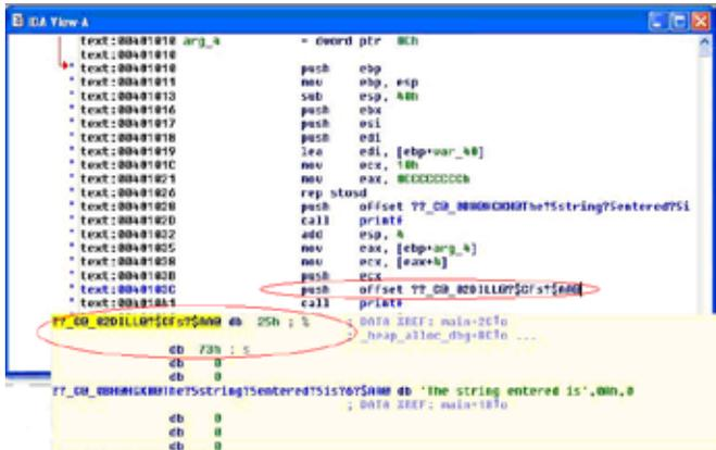
On the other hand, when the same code is compiled without "%s" as an argument, the variation in assembly is apparent. As seen below, there is no offset being pushed on the stack before calling printf.
