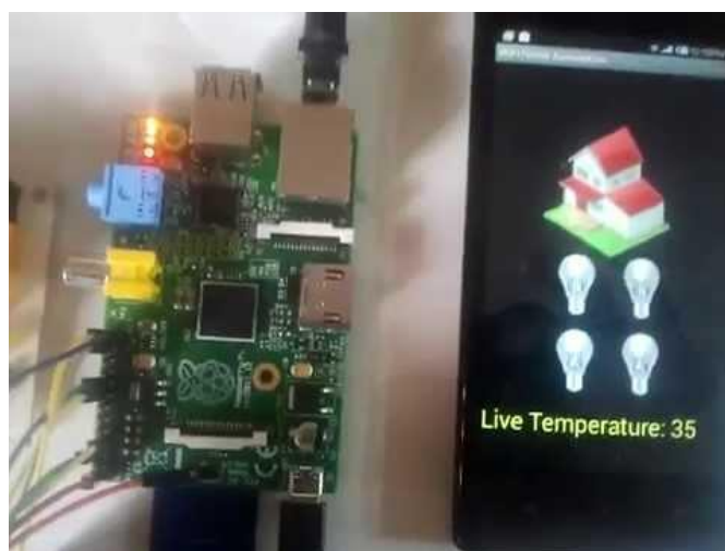
Figure 2-1 Android based Home automation using Raspberry Pi
