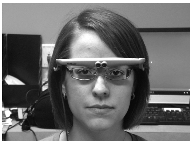
Figure 1: VisionPrint System: The subject wears a headset with sensors (as shown) and sits approximately 40 cm from the machine.
