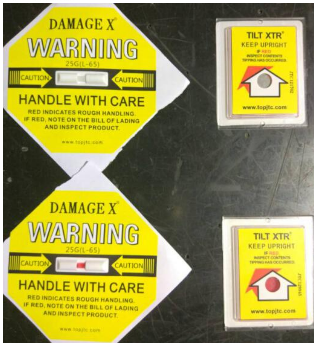
Figure 1-2 Changes of the Labels before and after Shock and Inclination
