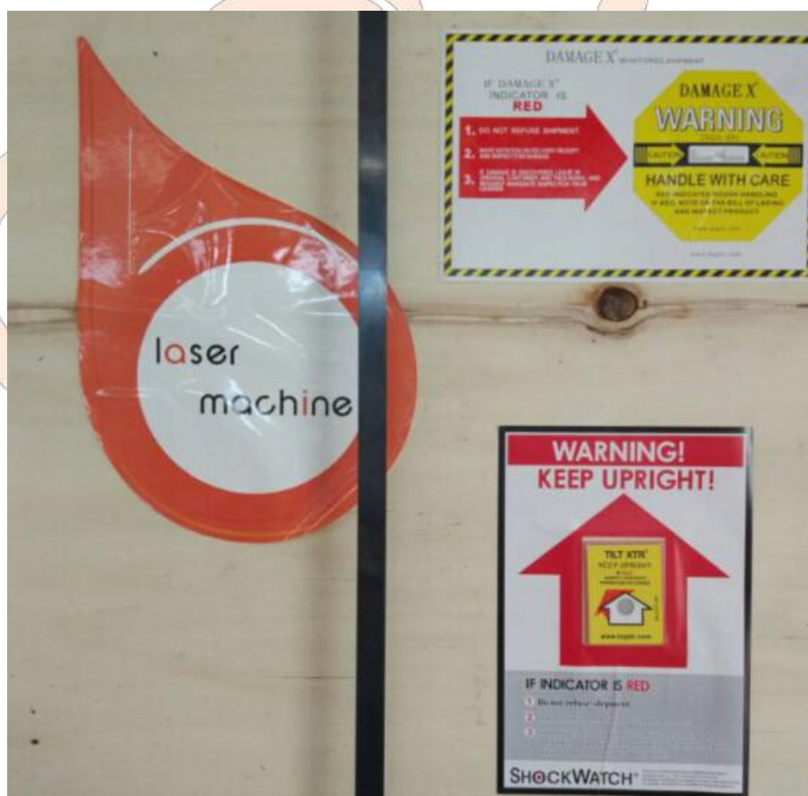
Figure 1-1 Shockproof and Inclination-proof Labels
