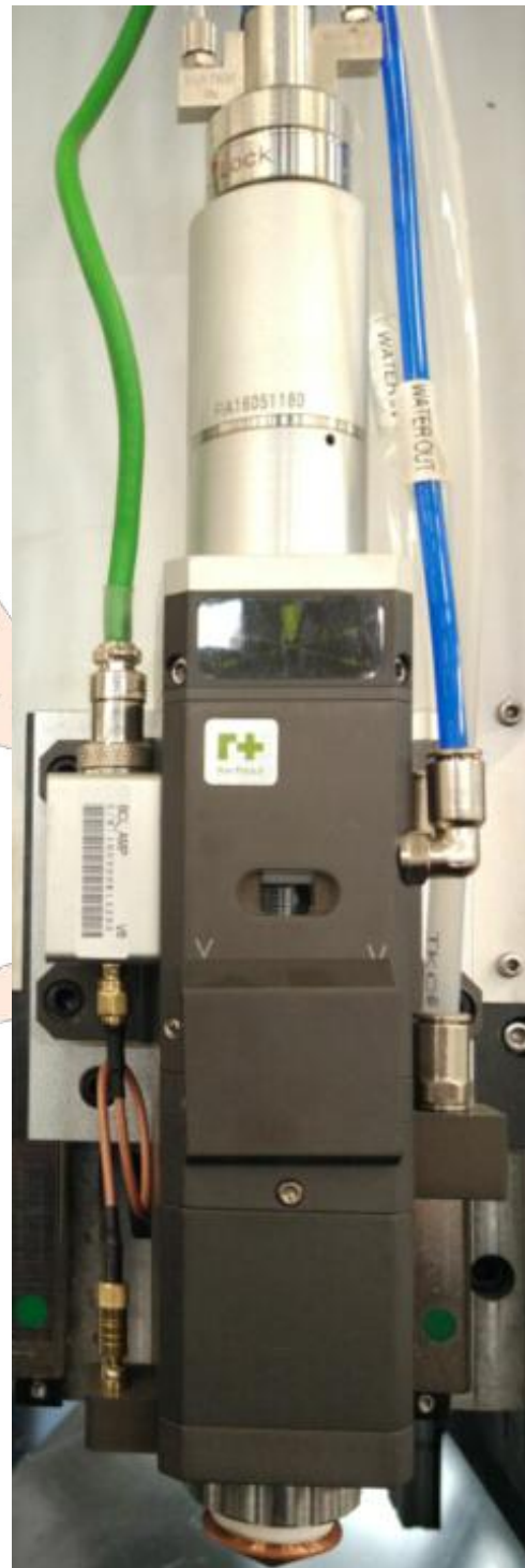
Figure 2-7 Example for Installation of Fiber Cutting Head
