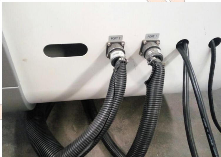
Figure 2-7 Example for Line Introduction of Control Cabinet
