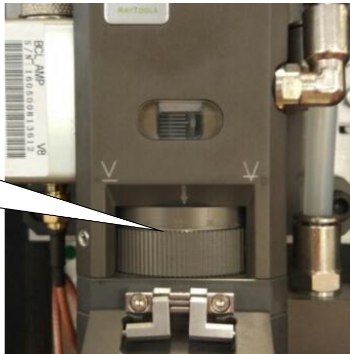
Figure 4-12 Setting Proper Focal Length
