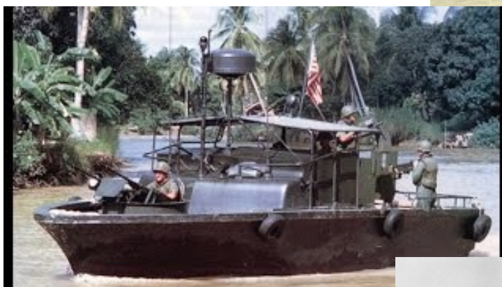
Patrol Boat, River. Length: 31 feet Beam: 11 feet, 9 inches, Displacement: 9 tons Speed: 35 knots Armament: Three .50-cal machine guns (two twinned, one single), one M60A machine gun and one MK-79 grenade launcher.
