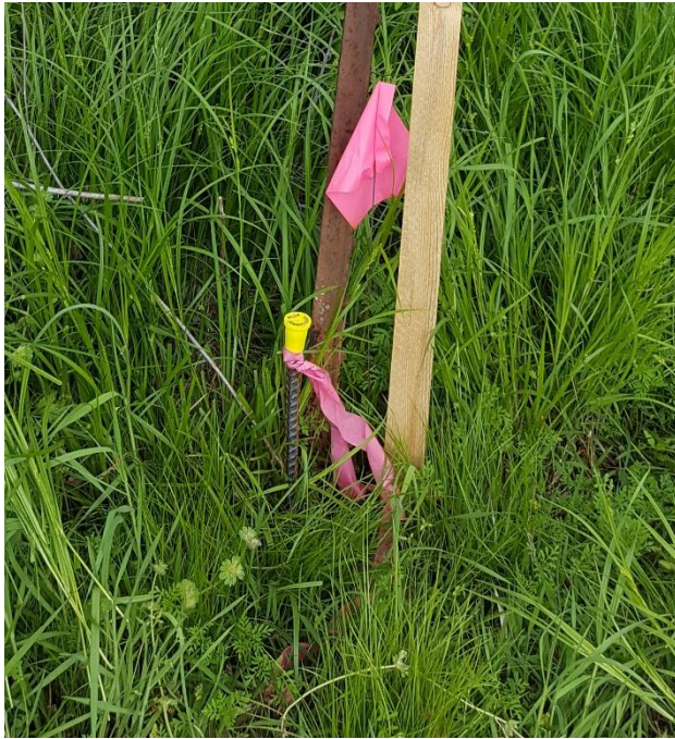
Figure 15. Parcel corner monument consisting of a 12 mm round iron peg
