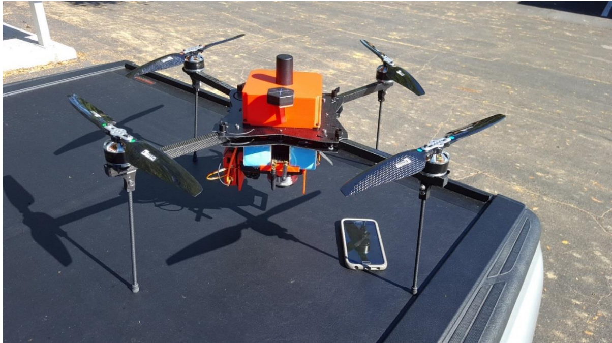
Figure 13. Survey quad copter equipped with a dual frequency V-Map GNSS receiver for accurate determination of CEPs
