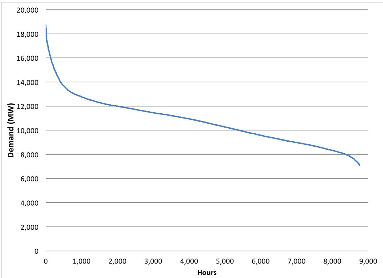
**FIGURE 38—LOAD DURATION CURVE FOR MICHIGAN UTILITIES FOR THE YEAR 2008. THE LOAD DURATION CURVE EXPRESSES HOW MANY HOURS DURING THE YEAR THAT THE SYSTEM EXPERIENCED DEMANDS ABOVE A PARTICULAR VALUE.**
