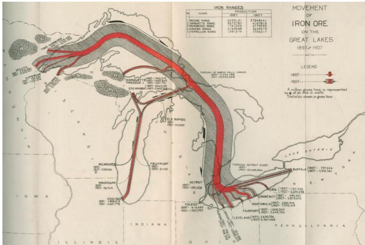
FIGURE 12—HISTORICAL DOCUMENT SHOWING MOVEMENT OF IRON ORE IN 1897 AND 1907<sup>55</sup>
