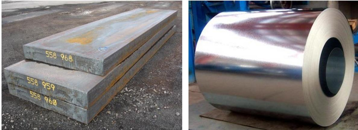
FIGURE 4—STEEL SLAB AND COIL<sup>12</sup>
