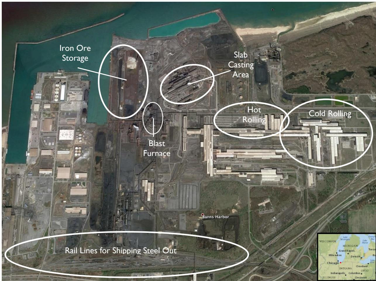
**FIGURE 28—BURNS HARBOR STEEL MILL**
