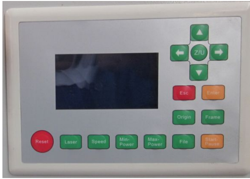
RD6442G control panel
