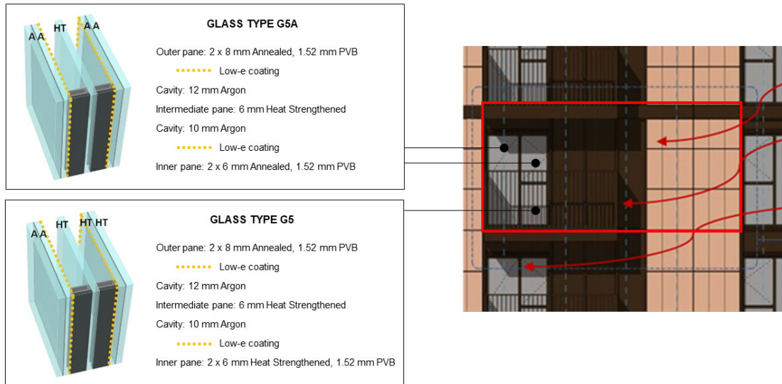
Figure 4 – Glass build-ups
