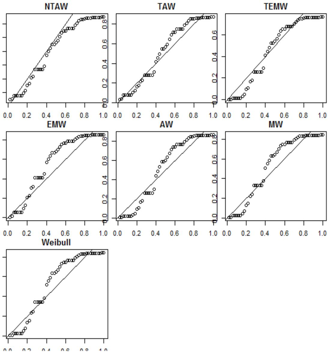
**Figure 10:** Probability plots for NTAW, TAW, TEMW, EMW, MW, Weibull, and AW of the data set 2.
