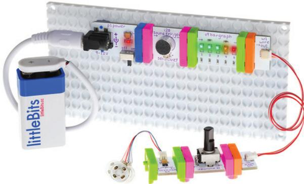
The mounting board allows students to keep their circuit intact and move it around with ease. Students snap together their littleBits circuit and press the feet of the Bits into the holes of the mounting board. Mounting boards also provide an effective way for students to store their circuits safely between work sessions.
