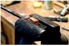
**6.** Use the appropriate size spacer for the material you will be using your tongs with and clamp into the vise to bend the second side of the box jaws.
