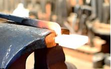
1. Place the flat jaw tong blank into the vise with the groove facing up and lined up with the edge of your vise. Then, use a twisting wrench to twist the jaw counter clockwise, when looking from the jaw down to the reins. 2. Repeat this process for the box jaw tong blank.
