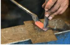
9. Cut excess length from the end of the flat jaw tong blank.
