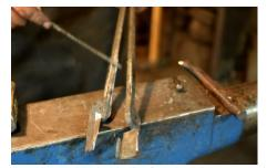
7. Drill the hole for the rivet.
