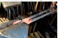
11. Make final adjustments by heating and squeezing/twisting as necessary to ensure the reins are lined up properly and will be comfortable to hold on to.
