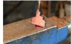
3. Use a cross peen hammer to thin the jaw of the box jaw tong blank.
