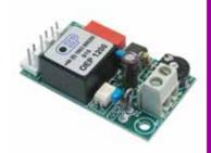
On-board amplifier for increasing the output volume of the internal loudspeaker or to connect an external loudspeaker.
