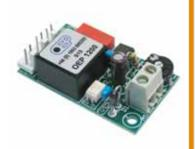
On-board amplifier for increasing the output volume of the internal loudspeaker or to connect an external loudspeaker.
