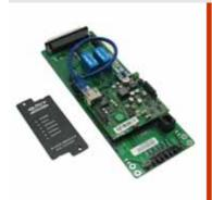
The IP-DAD (IP Digital Audio Decoder) is an audio decoder from IP network to analog signal and vice versa, converting the flow of digital data coming from the ASTRO PAVA system, through the redundant network, into an analog signal to feed the FPMD power amplifiers.
