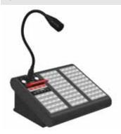
The DAP EN54-16 /100 Operator Console is a part of the EN54-16 certified Fitre P.A. System. It can manage various functions, including sending pre-recorded emergency announcements, sending live announcements via the gooseneck microphone, resetting system alarms, silencing emergency sound signals and other specific operations required by the EN54-16 standard.
