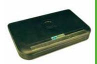
VoIP gateway with 2 FXS ports and 2 FXO ports
