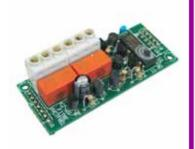
Card equipped with 2 relays (to switch door lock, lights, etc.) for remote or local control through programmable codes.
