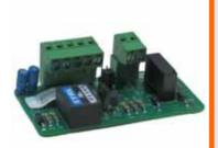
Speaker interface card for TAS360 VoIP and TAS2000 VoIP telephone set series allowing to connect an external amplified loudspeaker
