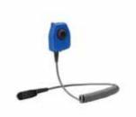
Nexus™ PTT adapter designed to be used with MT7H79P3E-50 ATEX headset; it enables users with 0-360 degree rotating clothing clip.
