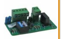
Speaker interface card for TAS360 VoIP and TAS2000 VoIP telephone set series allowing to connect an external amplified loudspeaker
