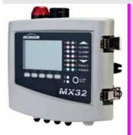
The MX 32 is a compact analog and digital low-profile controller that continuously monitors gas detection, including 4-20mA, dry logic input, MODBUS RS485 signal from compatible detectors.
