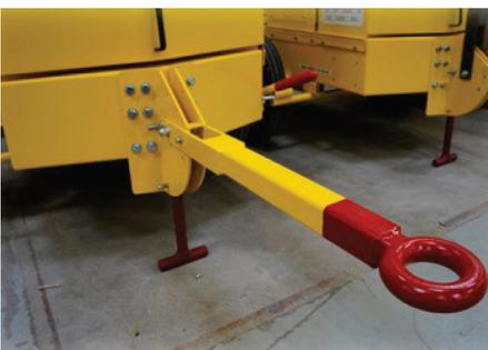
The BT400 NEX features the standard "long bar" and now we offer an optional swivel wheel kit for ease of maneuverability (below right). Tires have been standardized on all models to use tubeless tires and solid rims which are easier to maintain.
