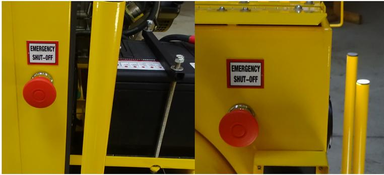
On the older model of heater it was possible for fuel delivery to continue to the combustion chamber in the absence of flame - now the cds “photo” sensor monitors and controls fuel delivery to ensure safe operation at all times. The heater is now CSA, UL, and O-TL certified. On newer models an emergency shut-off switch has been
