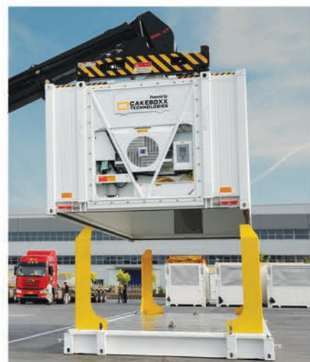
12' wide refrigerated CakeBoxx container for special temperature sensitive equipment
