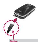
Please make sure that the LG logo faces down before inserting a charger or data cable into the charger port of your phone.
