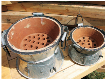
A traditional metal ‘jiko’ (the local word for cooking stoves) and the Kenya Ceramic Jiko. The most important modification is the introduction of a ceramic liner to conserve heat.
