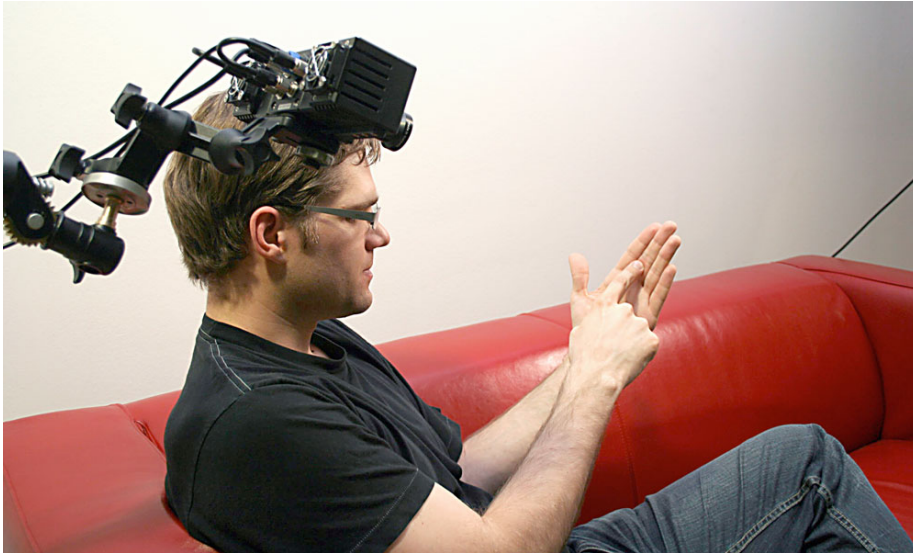
Figure 4.5: The prototype tracks input using a time-of-flight depth camera (PMD[vision] CamCube).
