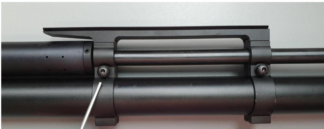
5. Now mark the upper side of the pressure tube on the side of the barrel. And then unscrew the pressure tube from the action.
