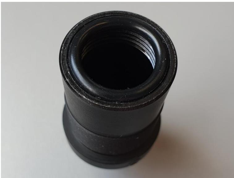
10. Now you can push the new regulator into the pressure tube. The scale label needs to be pointed towards the fill side of the pressure tube and the biggest diameter of the regulator will stand on the pressure tube's endcap. The small hole on the side of the regulator body needs to point upwards to the barrel side. (that is why you have marked the upper side of the tube)
