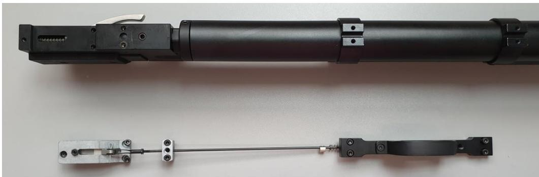
4. Loosen the two side bolts of the barrel- tube clamps
