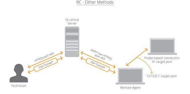
Remote control in SolarWinds N-central uses several layers of security. The outbound request model ensures that there are no inbound reports required.
