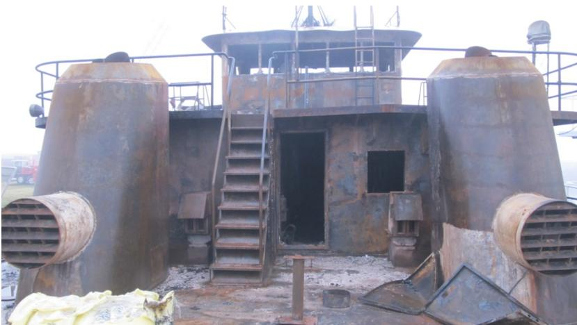
Aft side of *J.W. Herron* stacks, with engine room exhaust vents, post-fire.
