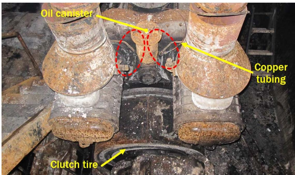
Aft side of starboard engine (viewed from above), with oil canister, remnants of clutch tire, and copper tubing identified. Red circles indicate areas where 1.5-inch stainless steel-braided rubber hoses were missing.
