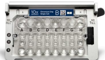
Recovery Well G indicates a reagent clog. Recovery Well C and E indicate a wetting failure. Recovery Wells B, D, and F are normal. Wells A and H contain 50% Glycerol Solution.
