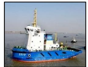
14.4m, a depth of 5.1m, a designed draft of 3.7m, a speed of 11.67kn, and a towing force of 42.1mt. On April 18, 2020, fifth patch
