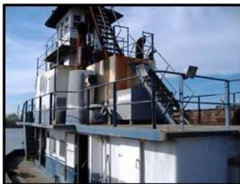
**File: TP14559 Push Boat:** 59.0' loa x 19.5' beam x 8.2' depth. Built in 1990 by Aiple Marine; Stillwater, MN. Rebuilt: 2002. U.S. flag. GRT: 77. Main Engines: 2 x CAT D348 **total 1,450BHP**. Last Overhauled: 2002. 2 - FP prop(s). Rebuilt 01/2002 by Alsem Industries. Genset(s): 2 - 40kW / GM3-71 (overhauled 2002). Quarters: 8. Galley. Totally rebuilt in 2002. Rewired. Upper Pilot house. Height of eye = 40'. **U.S. Gulf Coast. Prompt.**
