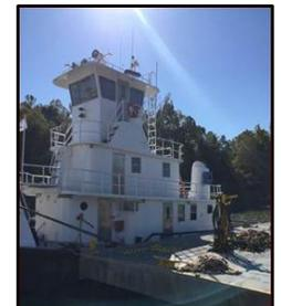
**File: TP07065 Push Boat:** 65.0' loa x 18.0' beam x 6.0' depth x **5.20' loaded draft**. Built in 1971 by South Shore Marine Shipyard; Holland, MI. U.S. flag. GRT: 65. Main Engines: 2 x Cummins N14 **total 700BHP**. Inland river pushboat. Retractable wheelhouse. Highest fixed point 15.6'. **U.S. Midwest.**
