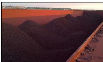
**File: HB19354 Hopper Barge – Inland (Up to 12 Available):** 193.7' loa x 54.4' beam x 12.0' depth. Built in 2007 by CIE; Paraguay. Foreign flag. Class: NKK NS RS BD HIDROVIA. Built under BV. **Dwt: 2,595mt. Hold Capacity: 3,700m3**. Twelve steel-built dry cargo barge rake and box type barges built between 2007 and 2009. No covers. **South America.**
