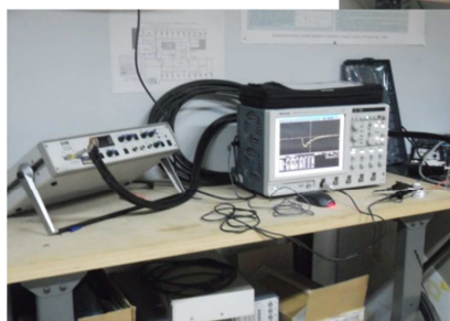
System for the generation of ultrashort high voltage electric pulses
