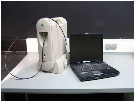
Portable spectroradiometer for field measurements (350-2500 nm spectral range)
