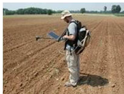
Measuring soil reflectance over agricultural land with a field spectroradiometer
