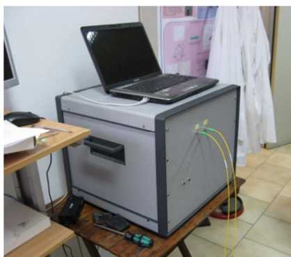
Prototype of a distributed sensors based on stimulated Brillouin scattering entirely developed at IREA
