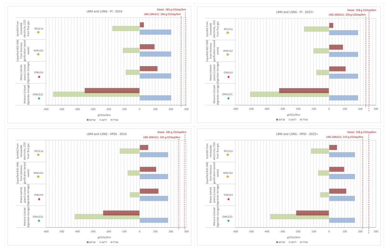
From a TTW perspective, the introduction of high-pressure direct injection (HPDI) engines is expected to lead to significant improvements.
