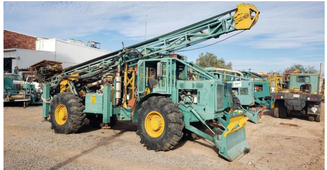
Skidder mounted drill rig capable of drilling to 1,000 meters and will be drilling diamond drill hole three in January, 2021
