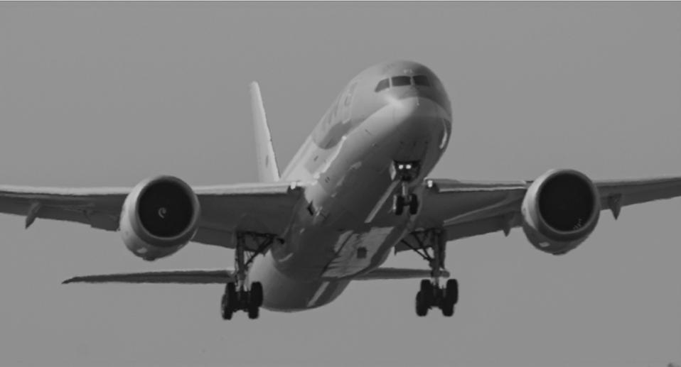
The Boeing 787 Dreamliner airframe is nearly 50% carbon fiber reinforced plastic and other advanced composites<sup>1</sup>
