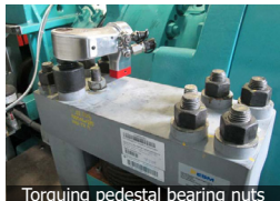
Torquing pedestal bearing nuts
