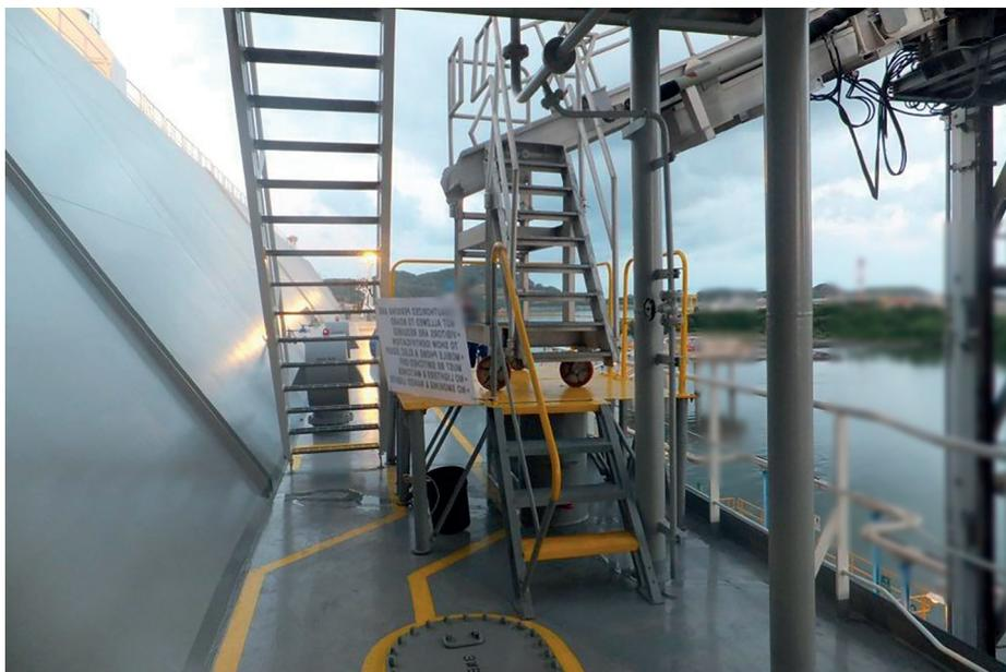
**Figure 8: Temporary portable platform over obstructive deck fittings and incorrect placement of gangway**
