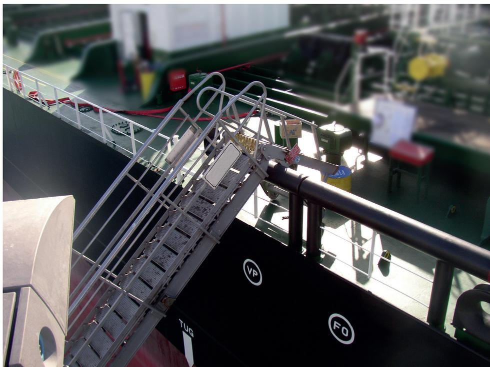
**Figure 5: Gangway not suitable for operational envelope**
