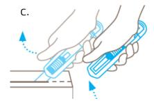
Thumbs up for a high degree of safety! As soon as you start cutting, remove your thumb from the slider, and the blade will disappear into the handle the moment it loses contact with the material you are cutting.
