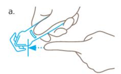
The blade is not open but concealed. Therefore, the cutting edge is shielded from you and the packaged goods, giving you a maximum degree of safety from cut injuries while cleverly protecting your products.
