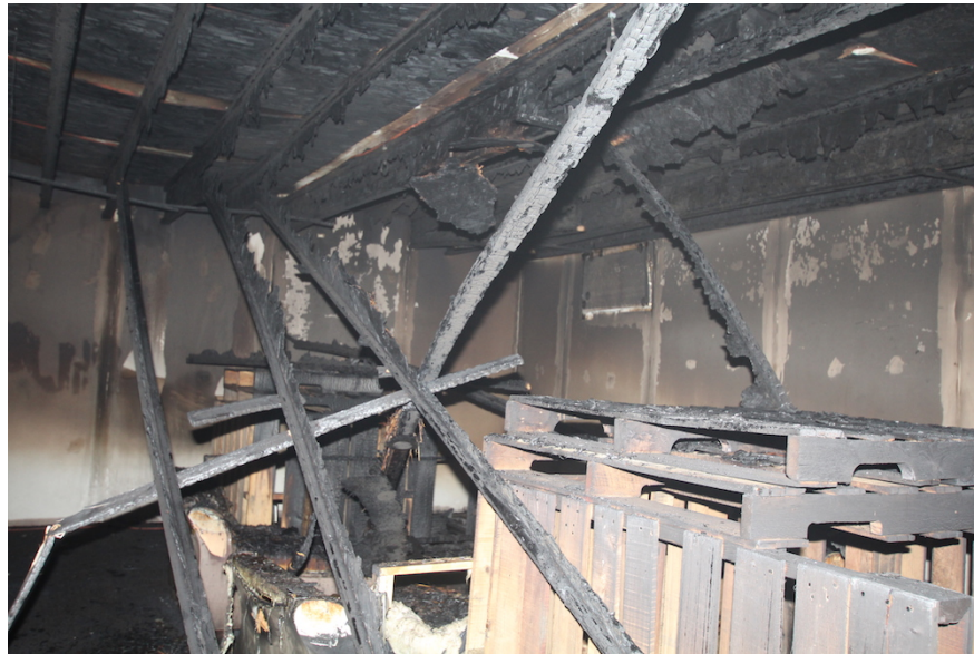
Figure 5.32: Photograph of the post-fire fuel packages on the ignition side.
