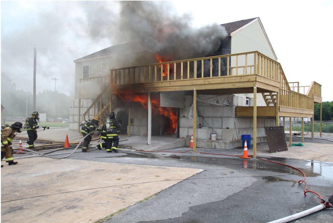
Figure 6.11: Photograph of flaming combustion extending outside of the structure indicating the presence of a ventilation-limited structure fire during Experiment 8.
