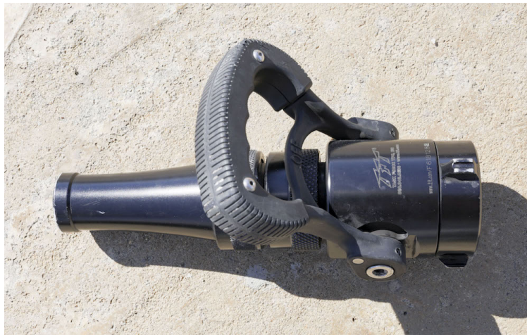
Figure 3.9: Example of smooth bore nozzle used in experiments.
