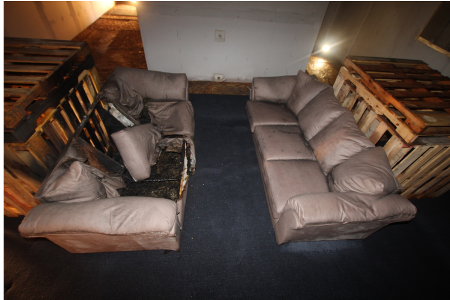
Figure 5.28: Photograph of the post-fire fuel packages on the ignition side.
