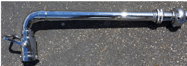
Figure 3.12: Example of Bresnan distributor nozzle used in experiments.
