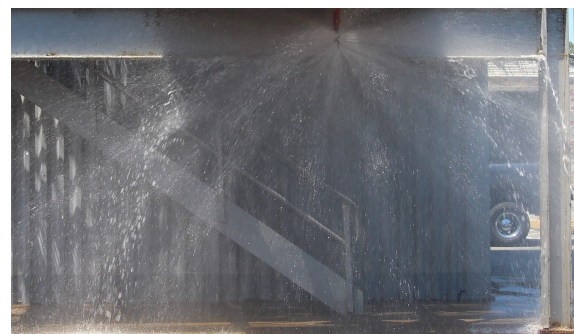
Figure 3.14: Examples of piercing nozzles: 125 gpm (left) and 150 gpm (right) spray patterns.
