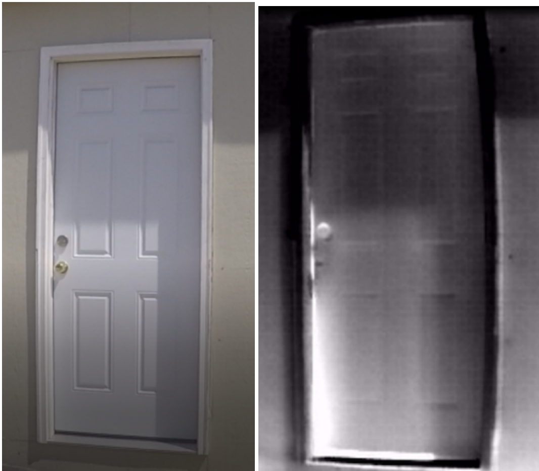
Figure 6.1: Comparison images ‘nothing showing’ of a closed door with a standard camera (left) and an IR camera (right).
