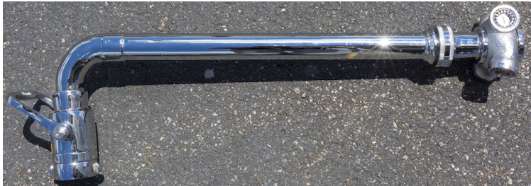
Figure 3.11: Example of cellar nozzle used in experiments.
