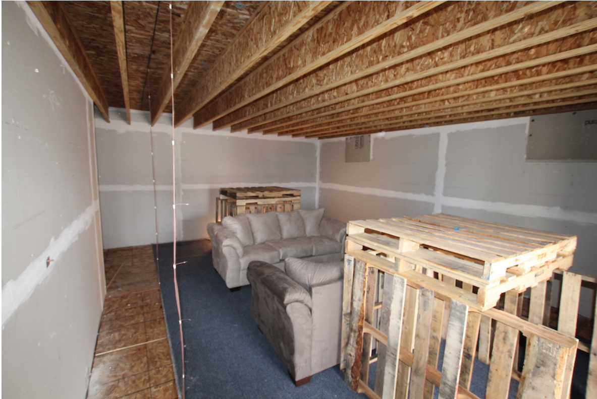
Figure 3.6: Photograph of installed fuel package on the west side of the basement.
