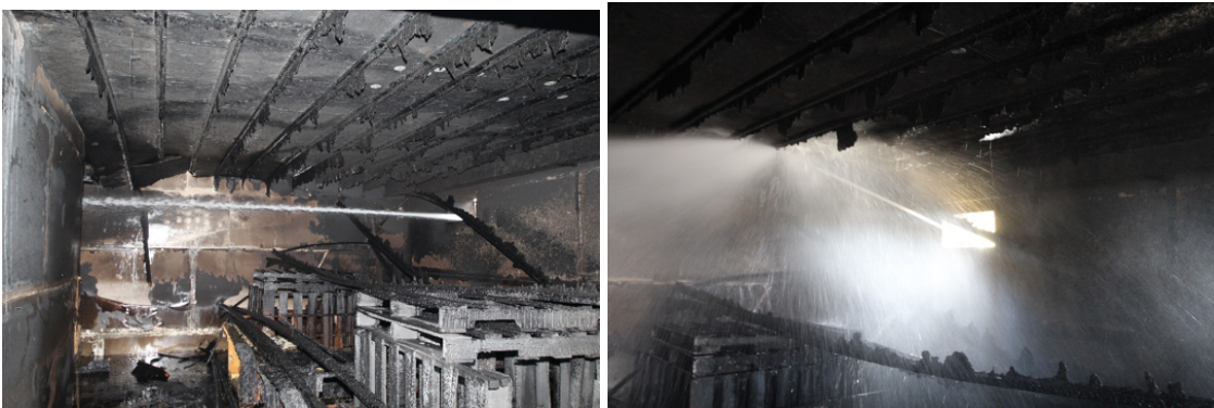
Figure 6.16: Photograph of straight stream through a window (left) and the broken stream produced by angling the stream off the ceiling (right).
