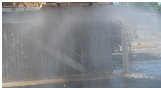
Figure 3.14: Examples of piercing nozzles: 125 gpm (left) and 150 gpm (right) spray patterns.
