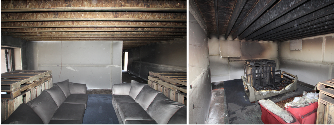
Figure 5.2: Photographs of the post-fire fuel packages on the non-ignition side (left) and ignition side (right).
