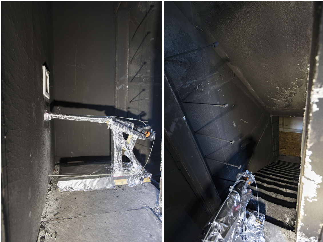
Figure 4.3: Photographs of the nozzle at the top of the stairwell from the side (left) and looking down the stairs (right) in Experiment 12.
