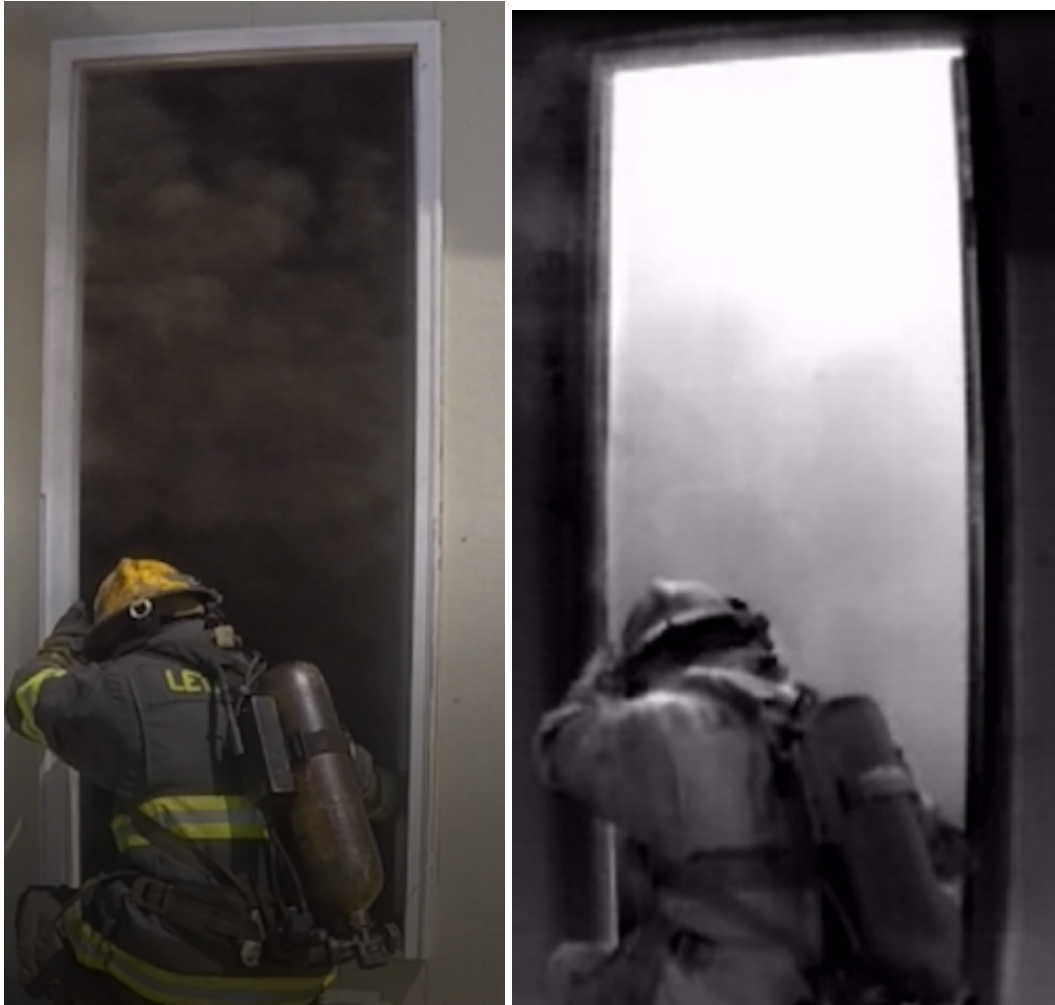
Figure 6.2: Comparison images of a open door with a standard camera (left) and an IR camera (right).
