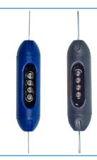
The frequency of the flashing LEDs indicates the voltage level on the fence. The longer the period between flashes, the lower the voltage on the fence. The intensity of the light remains the same so it can be seen from far irrespective of the fence voltage. It is installed between the earth and live wire to indicate the status and condition of the fence for peace of mind.
