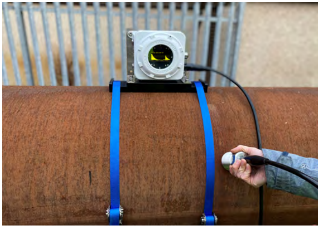
Figure 1. Dual-functionality ultrasonic pig signaller with locating function.
