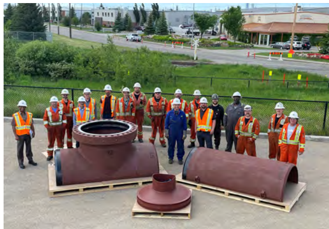
Figure 4. 48 in. fitting and completion plug manufacture (Edmonton, Canada).
