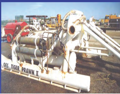
World's deepest water post trencher sled 1200 ft
