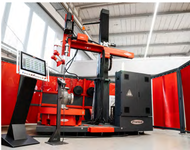
Figure 4. Compact Cladding Cell with rotating positioner, HMI-T21 system controls, and remote control.
