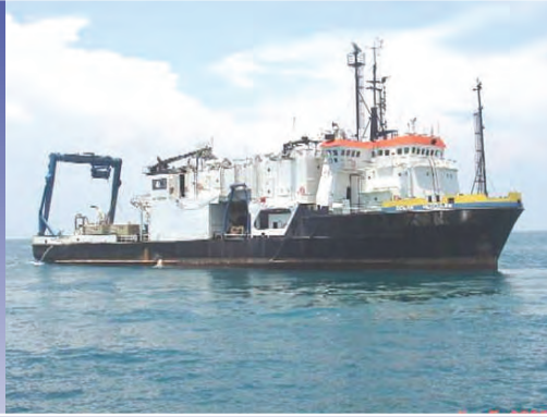
Typical Dynamic Positioned Vessel during Trenching (Lead Keel Machine)
