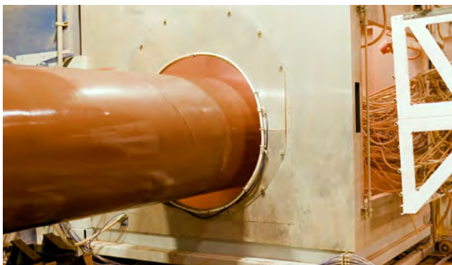
Sherwin-Williams. A moisture- and abrasion-resistant overcoat fusion-bonded epoxy (FBE) layer of Pipeclad® 2060 MRO is applied immediately after a base anti-corrosion FBE layer of Pipeclad 2000, allowing the two powdered coatings to crosslink before curing to form an extremely durable protective coating system for buried pipelines.
