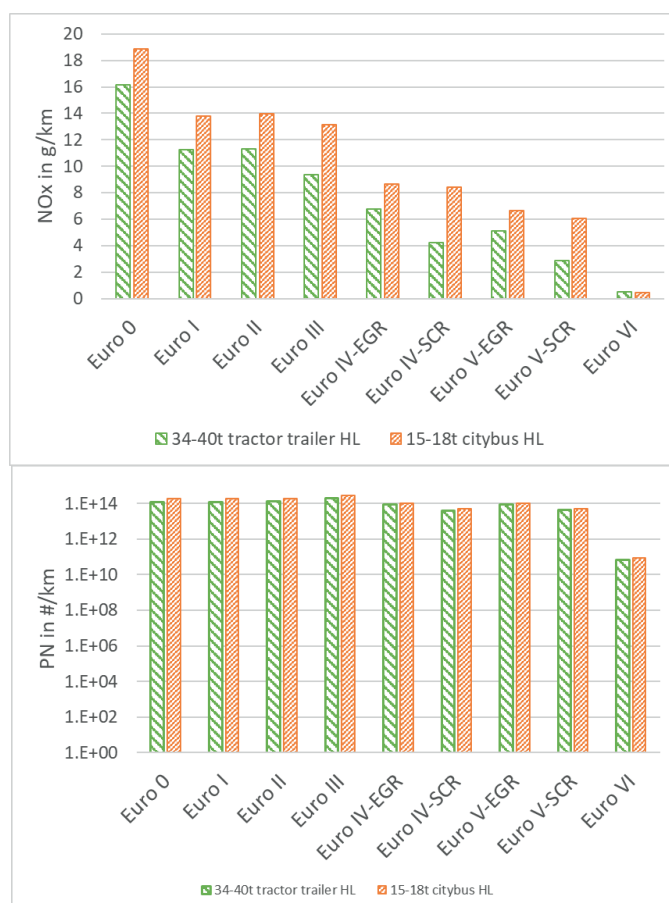
Figure 5-1: Average hot NOx (upper) and PN (lower) emission factors for a HDV tractor semi-trailer combination 34–40t and for a city bus (15–18t class) from HBEFA 4.1 for 50 000 km cumulated mileage for their corresponding German traffic situation mix 11
