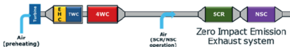
Figure 7-1: Exhaust layout of AVL petrol demonstrator (Kapus, 2020; Kapus et al., 2020)
