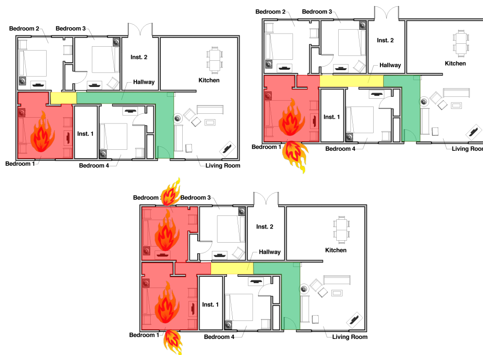
Figure 7.26: Thermal conditions during the three ventilation configurations, no vent Experiment 1 (left), single vent Experiment 12 (right) and two vent, Experiment 17 (bottom) just prior to hall suppression crew arrival time. Color conditions represent operating zones per Utech [31] where green is routine, yellow is ordinary, and red is emergency.
