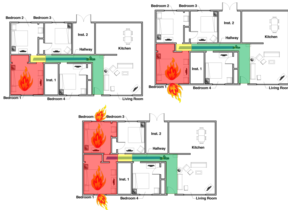
Figure 7.27: Thermal conditions during the three ventilation configurations, no vent Experiment 4 (left), single vent Experiment 7 (right) and two vent, Experiment 13 (bottom) 10 seconds after hallway suppression while conducting an interior attack. Color conditions represent operating zones per Utech [31] where green is routine, yellow is ordinary, and red is emergency.
