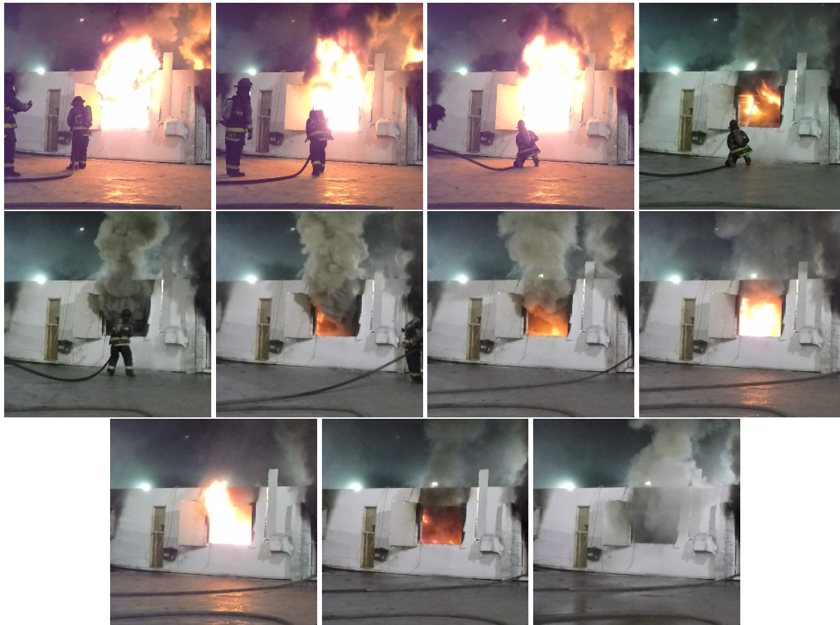
Figure 7.20: Image sequence of transitional attack from 10 seconds prior to water application (top left) through suppression 40 seconds after initial suppression (bottom right).
