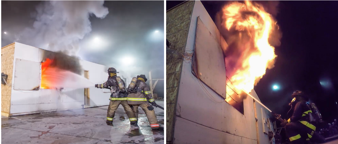
Figure 7.18: Examples of the potential to change the flow path based on the application of water from the exterior. The narrow fog (left) blocks the opening and entrains air increasing the pressure in the room, the solid stream (right) does not affect the flow path.
