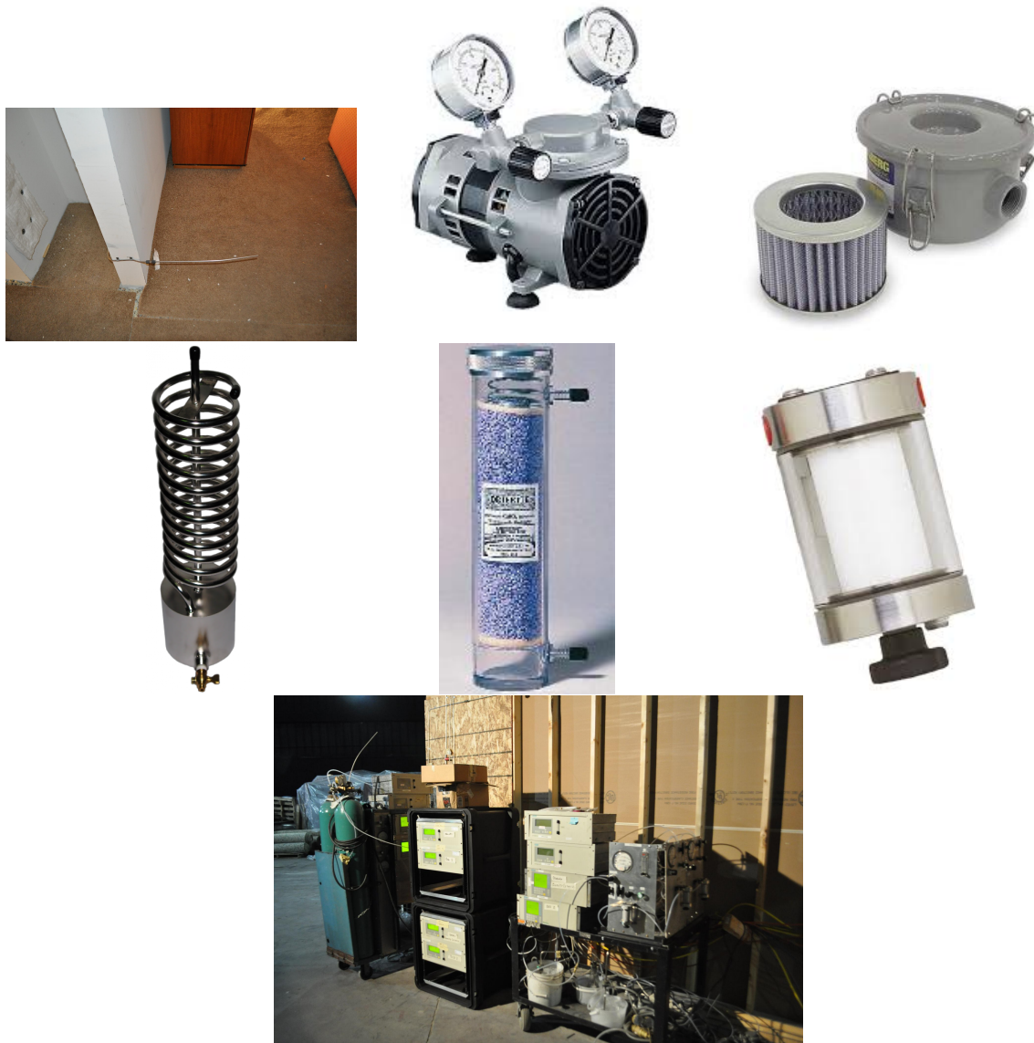
Figure 4.21: Gas Analyzer Configuration, Gas Sample Point (Top Left), Vacuum Pump - Cole Palmer L-79200-30 (Top Center), Course Filter - Solberg 842 (Top Right), Condensing Tube (Middle Left), Drierite Tube (Middle Center), Fine Filter - Perma Pure FF-250-SG-2.5G (Middle Right), Gas Analyzer Setup (Bottom)
