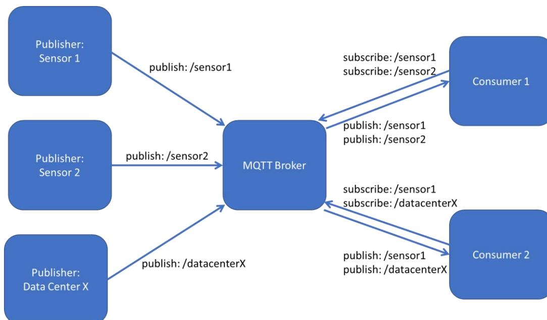
**Figure 5: Schematic overview of MQTT**
