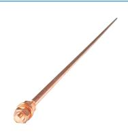
The copper cladded earth spike or stake is used to earth the electric fence system. A minimum of 3 earth spikes must be knock into the ground near the electric fence at a minimum of 1.5 m apart. Connect these earth spikes to the energizer or the fence using the high tension insulated cable (HT). In areas where earthing conditions are bad you may be required to add a few more earth spikes/stakes along the fence line and connect these back to the energiser.
