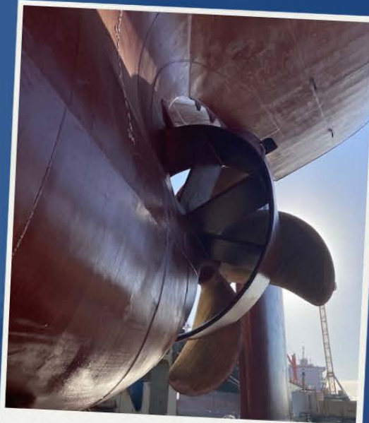
Becker Mewis Duct Installation
