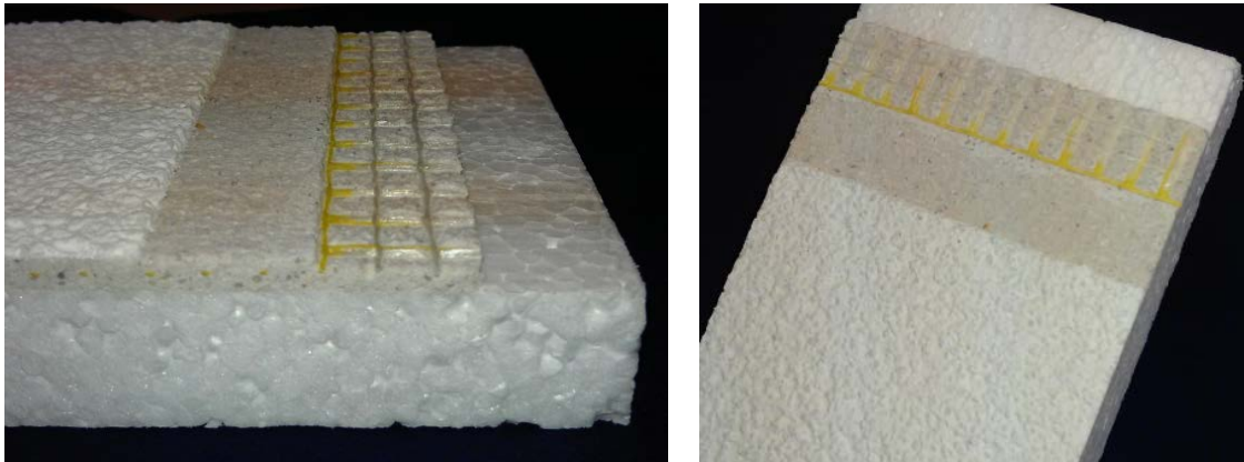
Figure 4.33 – Thin coat render build-up
