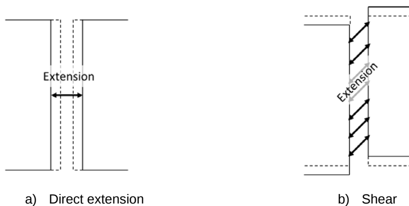
Figure 6.5.8 – Movement at joints
