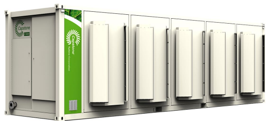
A C1000R Microturbine provides up to 1 MW of electrical power and contains 5 microturbine engines.
