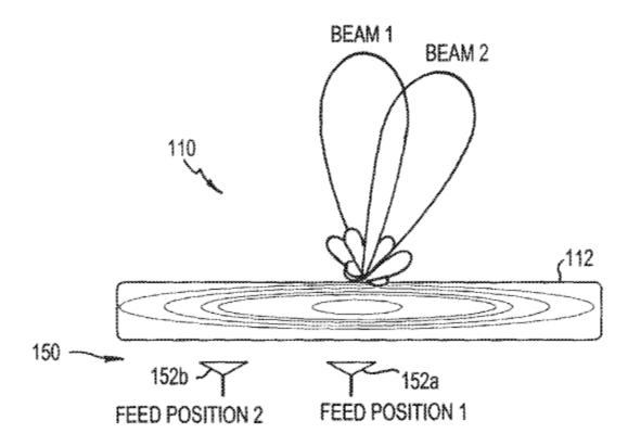
Figure 2, reproduced above, shows feeds 152a and 152b that direct electromagnetic energy through lens 112 (in lens set 110) in patterns as
