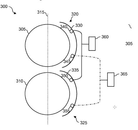
Figure 3, reproduced above, illustrates antenna system 300 with RF elements 340, 345 and 350, 355 movable along curved tracks 320 and 335 of adjacent surfaces of each lens 305 and 310, respectively. Ex. 1002, 8:1–20. Control mechanism 360, which includes a phase shifter, controls the phase and positions of RF elements 340, 350. *Id.* at 8:28–37. Similarly, control mechanism 365, which also includes a phase shifter, controls the phase and position of RF elements 345, 355. *Id.*
