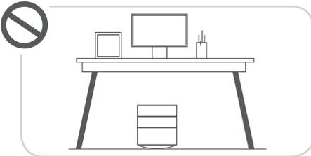
DO NOT PLACE UNDER A TABLE OR WHERE THE AIR OUTLET WILL BE BLOCKED
