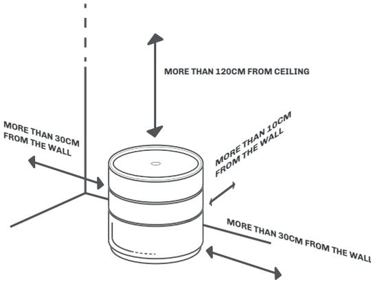
For maximum performance and reliability, place BRID at a suitable distance from the wall. Do not obstruct BRID's fan located at the base of the product. It is important not to block the airflow.
