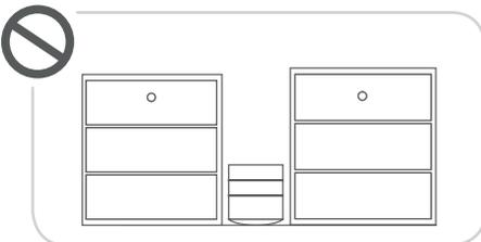
DO NOT PLACE BRID BETWEEN LARGE OBJECTS THAT COULD LIMIT THE AIRFLOW
