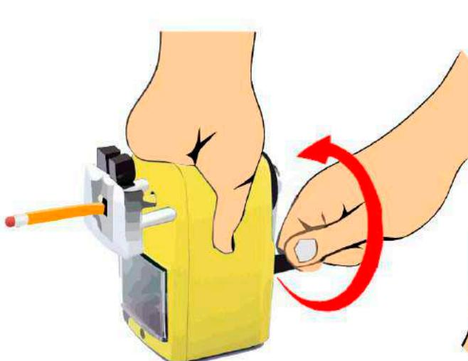
3. Place one hand on top of the sharpener to hold it secure. Do not hold onto the pencil while sharpening. Turn the handle clockwise to sharpen. The face will pull the pencil in automatically. The handle will spin freely once the pencil is fully sharpened.
