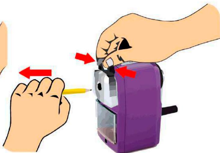
3. Place one hand on top of the sharpener to hold it secure. Do not hold onto the pencil while sharpening. Turn the handle clockwise to sharpen. The face will pull the pencil in automatically. The handle will spin freely once the pencil is fully sharpened.
