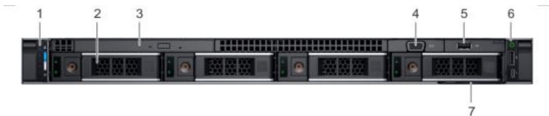
Figure 4.13: PILATUS3 X 100K-M detector control unit as seen from the front.
