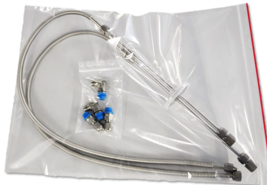
Figure 4.12: Picture of the optional PILATUS3 X 100K-M cooling vacuum feedthrough set with tubes through a standard DN40ISO-KF flange, and straight and elbow connectors for the detector head.
